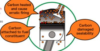
Accumulated carbon through driving will degrade engine performance CN101 cleans engine combustion system by quick operation to improve engine condition
