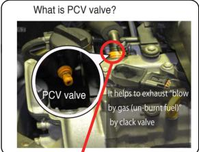
PCV valve circulates blow by gas which came out from a tiny space of piston and cylinder into the intake pipe again.
